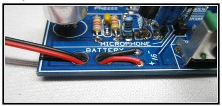
In case you haven't seen this before, running the 9v battery snap leads down and then back up a pair of holes makes a nice strain relief to keep the fragile leads from breaking.
